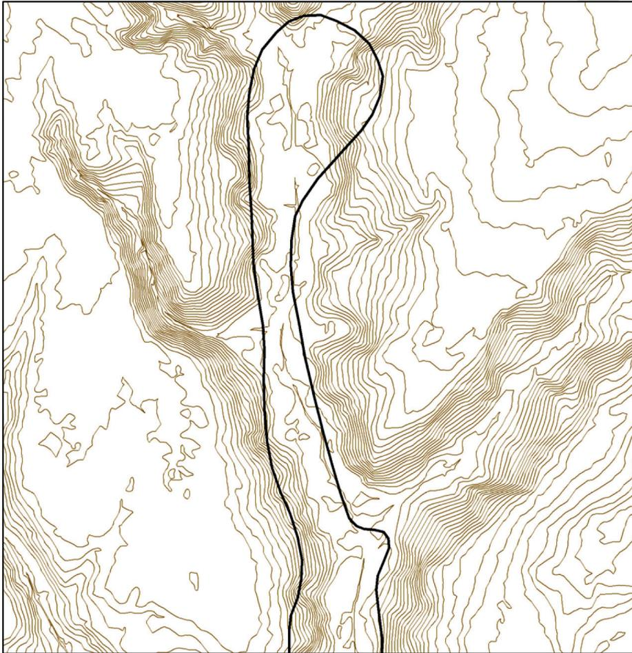
**Figure 7. Un-numbered A Zone, shown with the black line, against 2-foot contours derived from LiDAR, shown by the lighter lines. (MEGIS, 2009.)**
