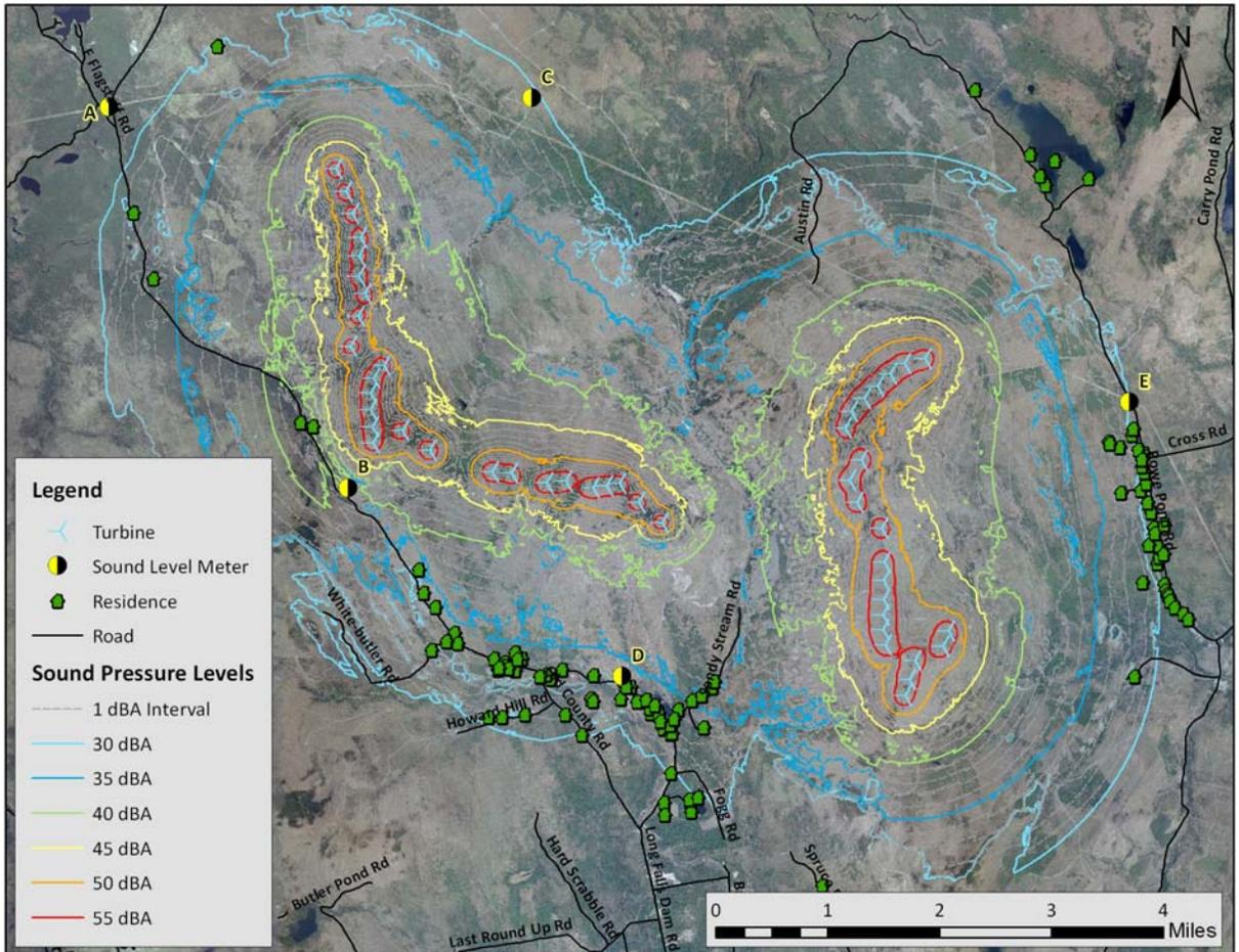
Figure B22: A-weighted Overall Modeled Sound Pressure Levels (dBA) from the Highland Wind Project at Maximum-Rated Sound Power, Scenario 2 (Siemens 101, Vestas V90)
