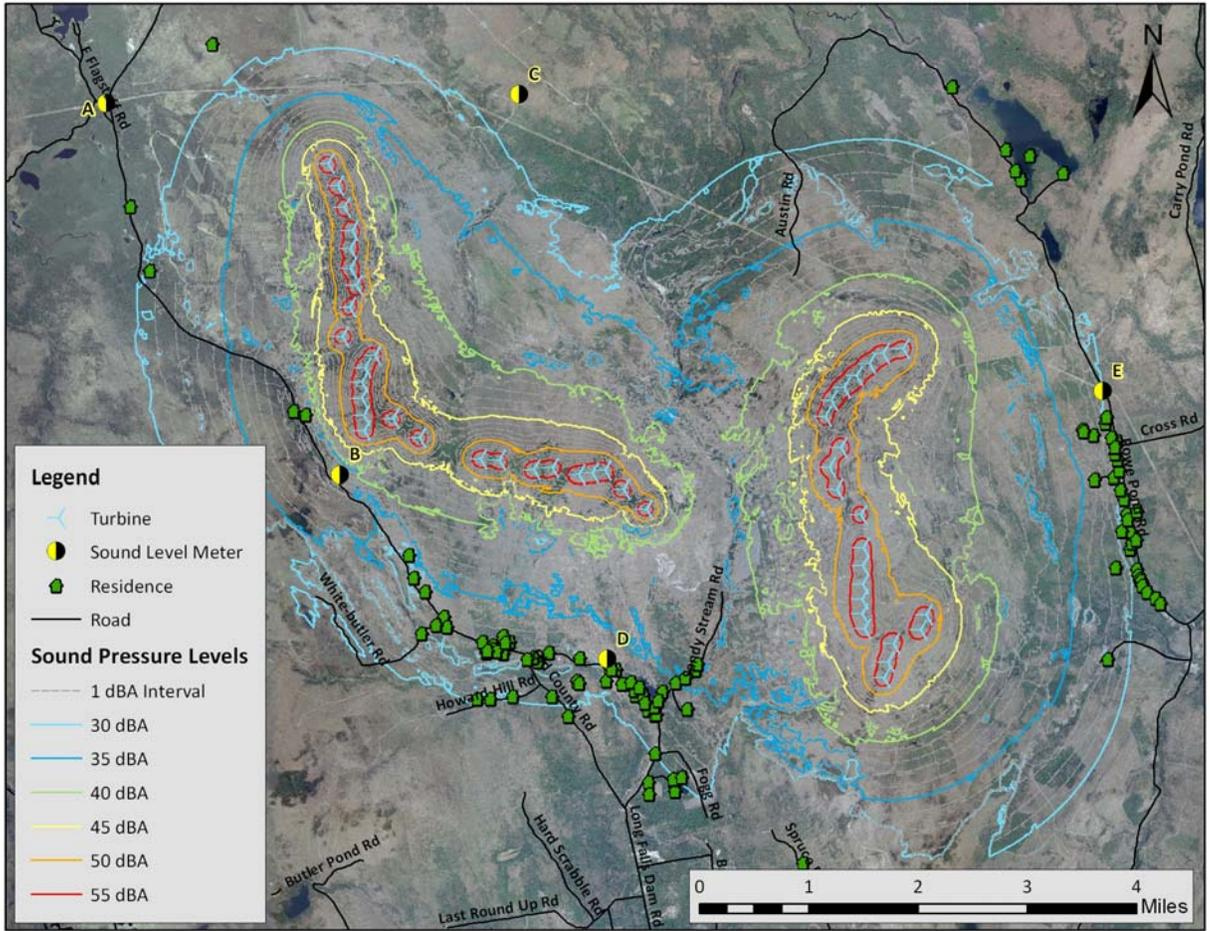
Figure B55: A-weighted Overall Modeled Sound Pressure Levels (dBA) from the Highland Wind Project at Maximum-Rated Sound Power, Scenario 5 (Vestas V90, Siemens S93)
