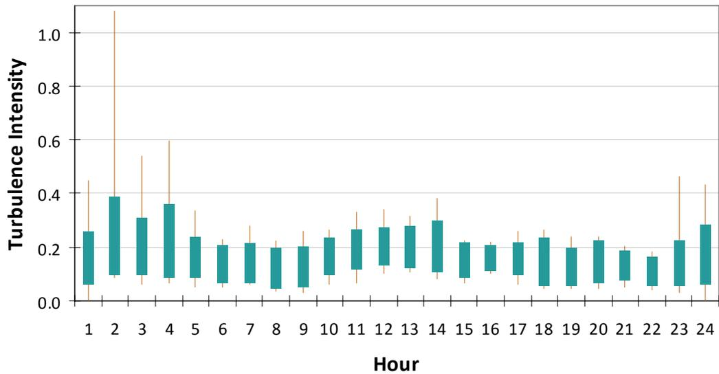
Figure D8: Turbulence Intensity by Hour at Witham Mountain Met Tower, 48.5m Anemometer Height
