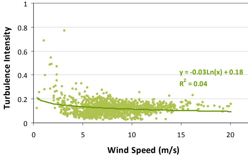
Figure D2: Turbulence Intensity by Wind Speed at Stewart Mountain Met Tower, 40m Anemometer Height
