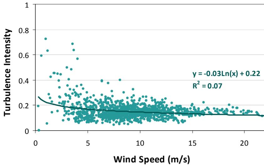
Figure D5: Turbulence Intensity by Wind Speed at Burnt Hill Met Tower, 48.5m Anemometer Height
