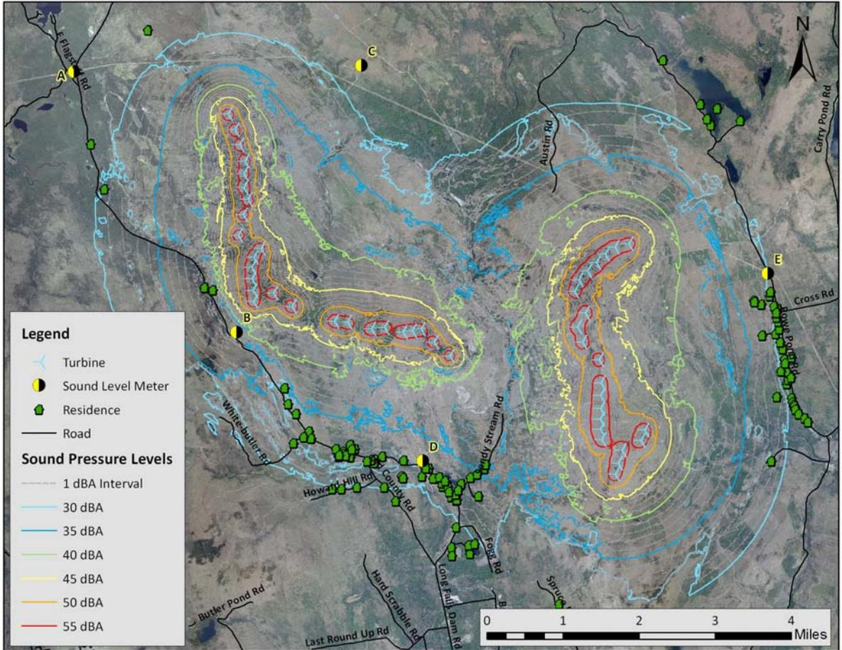
Figure B33: A-weighted Overall Modeled Sound Pressure Levels (dBA) from the Highland Wind Project at Maximum-Rated Sound Power, Scenario 3 (GE 2.5xl, Siemens S93)
