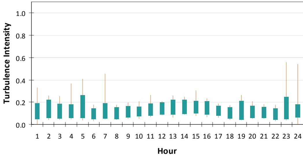
Figure D9: Turbulence Intensity by Hour at Witham Mountain Met Tower, 25m Anemometer Height
