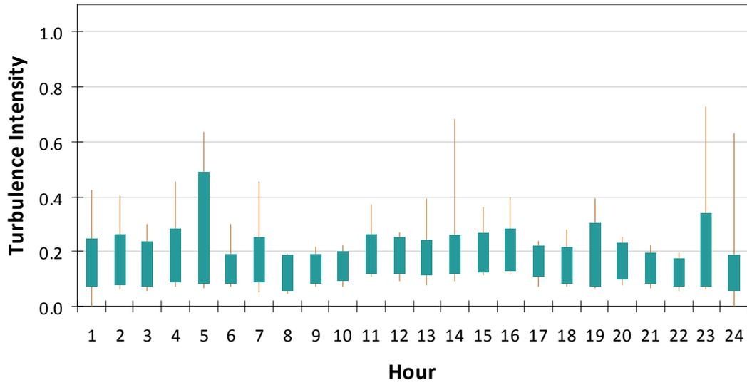
Figure D9: Turbulence Intensity by Hour at Burnt Hill Met Tower, 48.5m Anemometer Height
