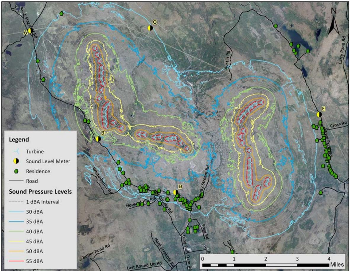
Figure B66: A-weighted Overall Modeled Sound Pressure Levels (dBA) from the Highland Wind Project at Maximum-Rated Sound Power, Scenario 6 (Vestas V90, Vestas V90)
