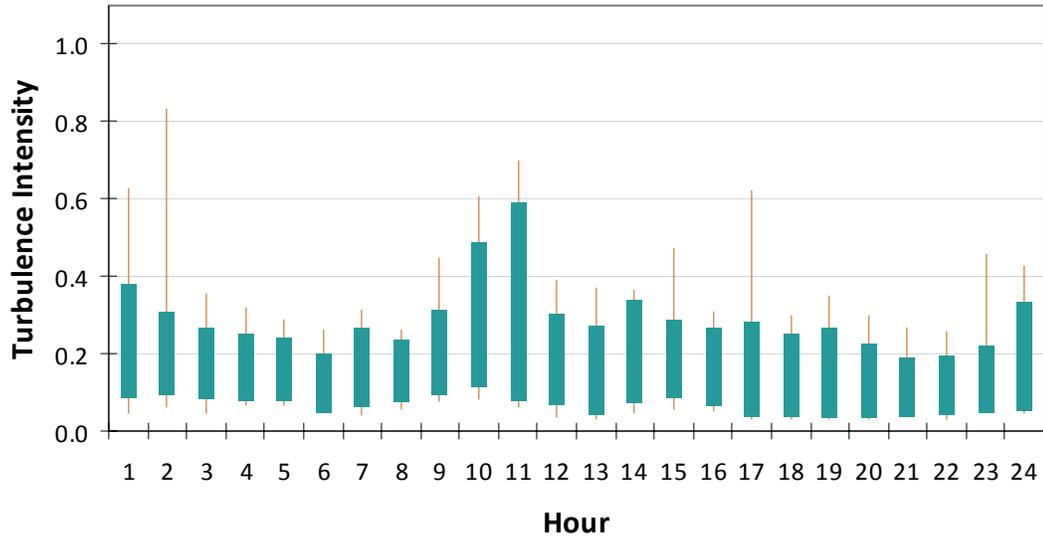
Figure D10: Turbulence Intensity by Hour at Burnt Hill Met Tower, 25m Anemometer Height
