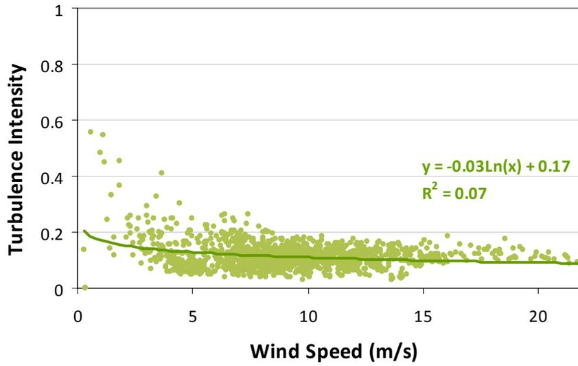
Figure D4: Turbulence Intensity by Wind Speed at Witham Mountain Met Tower, 25m Anemometer Height
