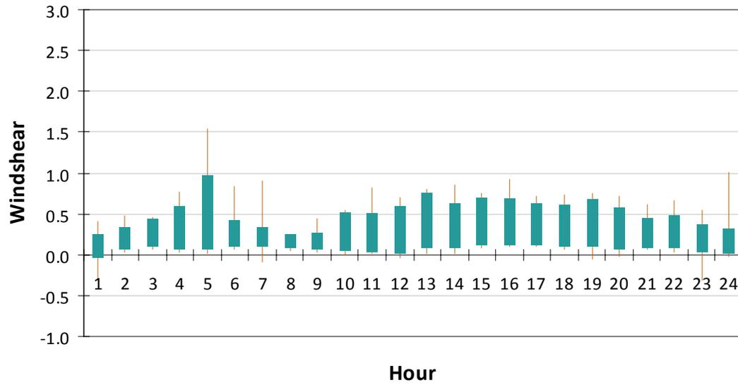
Figure D13: Windshear by Hour at Burnt Hill Met Tower, 80m Anemometer Height
