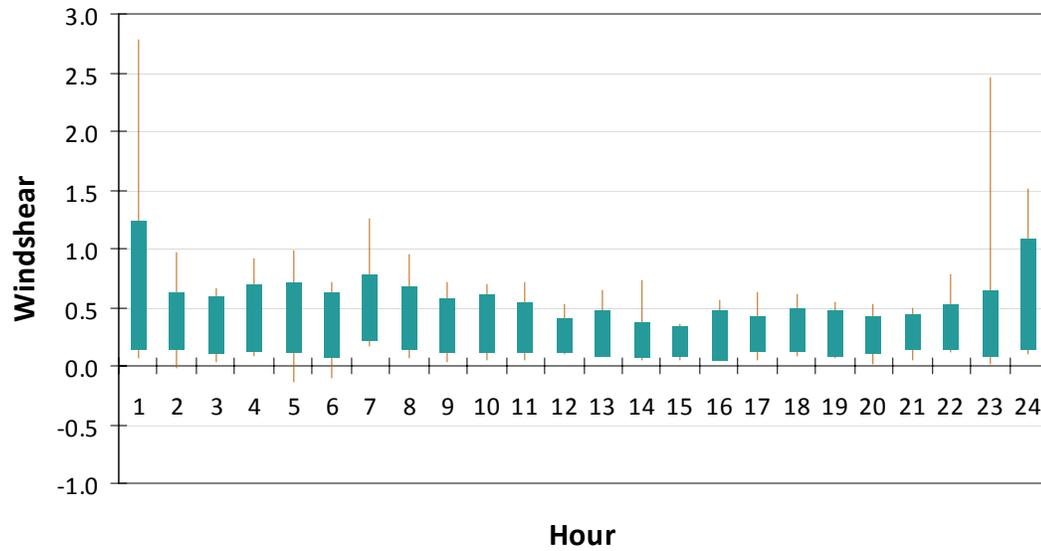
Figure D12: Windshear by Hour at Witham Mountain Met Tower, 80m Anemometer Height
