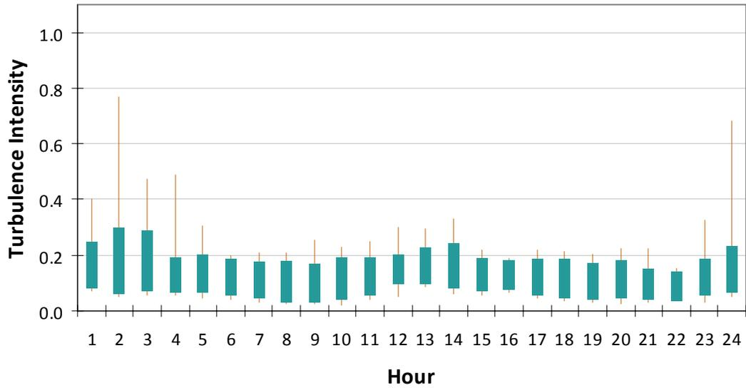
Figure D8: Turbulence Intensity by Hour at Stewart Mountain Met Tower, 40m Anemometer Height
