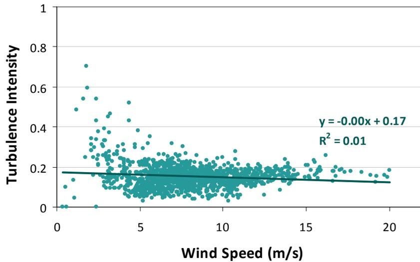
Figure D3: Turbulence Intensity by Wind Speed at Witham Mountain Met Tower, 48.5m Anemometer Height
