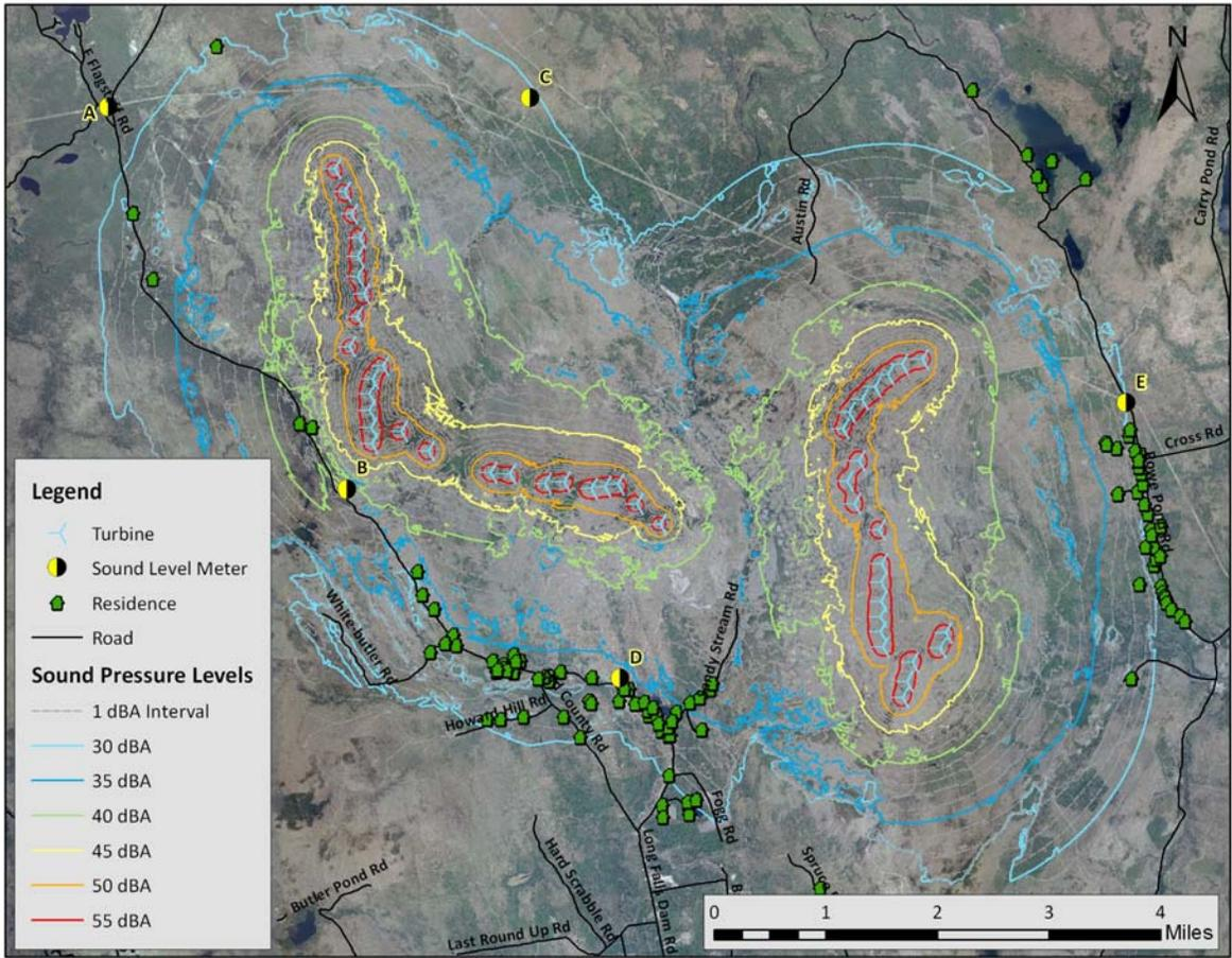
Figure B44: A-weighted Overall Modeled Sound Pressure Levels (dBA) from the Highland Wind Project at Maximum-Rated Sound Power, Scenario 4 (GE 2.5xl, Vestas V90)
