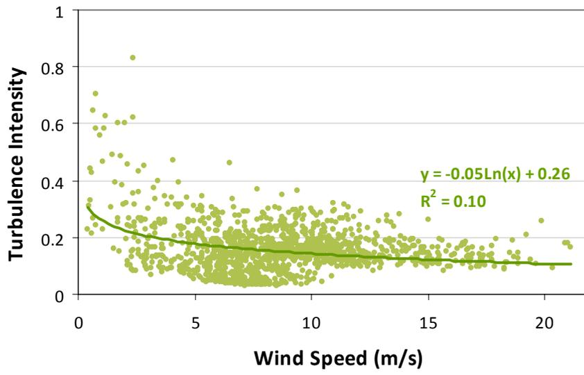
Figure D6: Turbulence Intensity by Wind Speed at Burnt Hill Met Tower, 25m Anemometer Height
