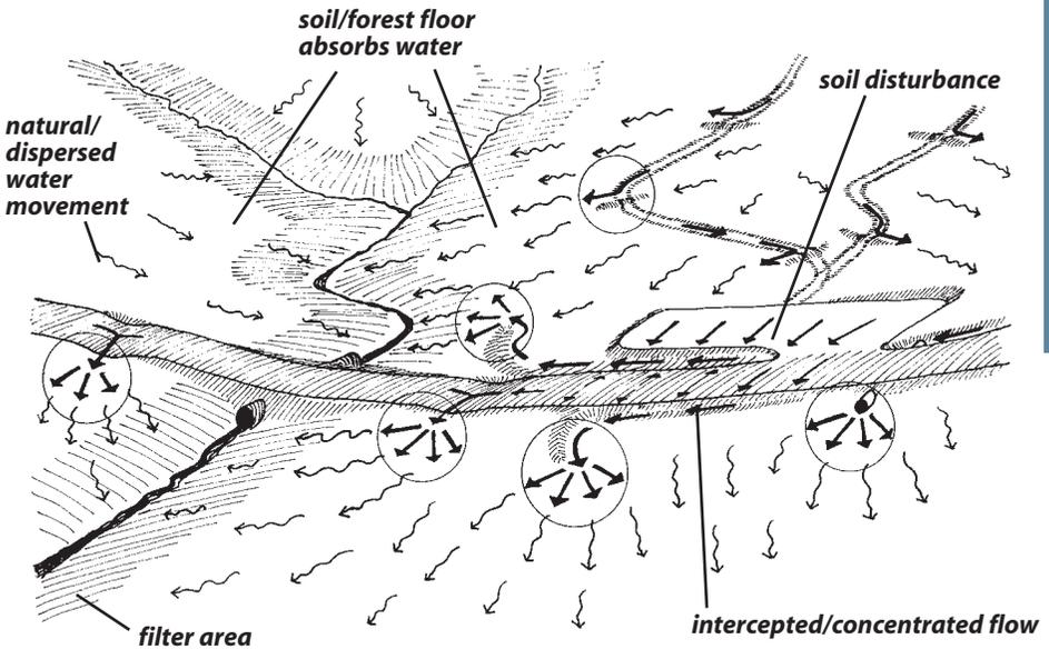
*One way BMPs minimize impacts to water quality is by dispersing concentrated water flow. Circles indicate where BMPs disperse flow to the undisturbed forest floor.*
