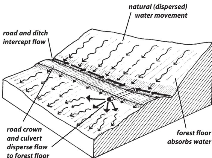
*Harvesting operations intercept natural water movement and concentrate it in ditches or on the road/trail surface.*
