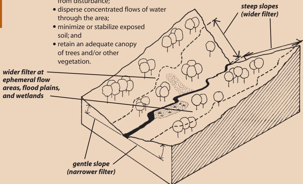
*The minimum filter width varies with slope and site conditions.*
