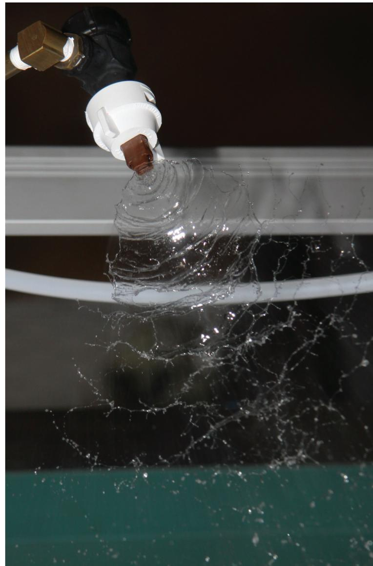
*(Left) This photo shows a spray that does not contain a drift suppressing adjuvant. (Right) This photo shows a spray that does contain a drift suppressing adjuvant. Notice how the spray with the adjuvant remains in a “sheet” longer.*
