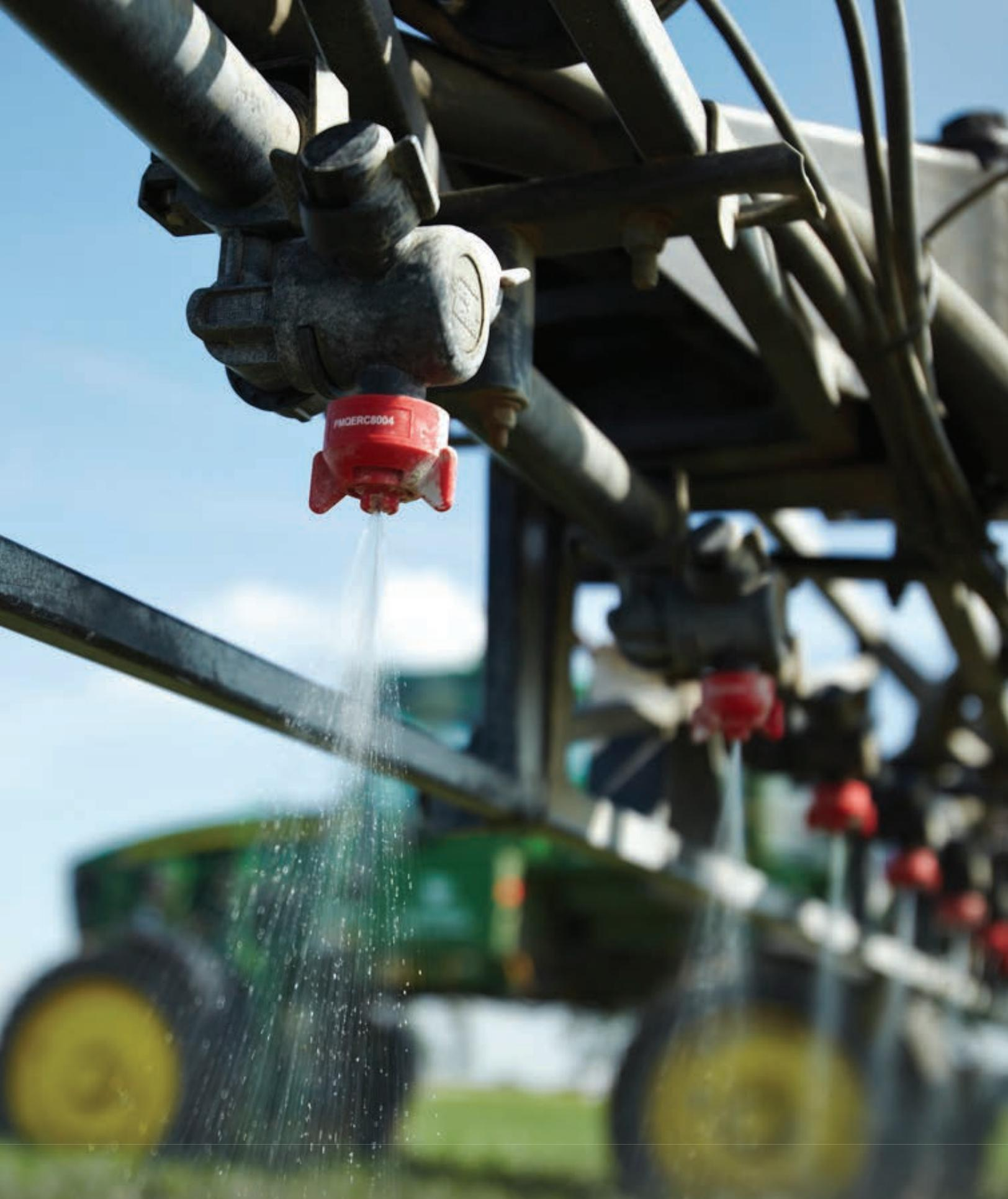
*When a nozzle emits a spray, the solution goes from a film, to segments, to spray droplets.
