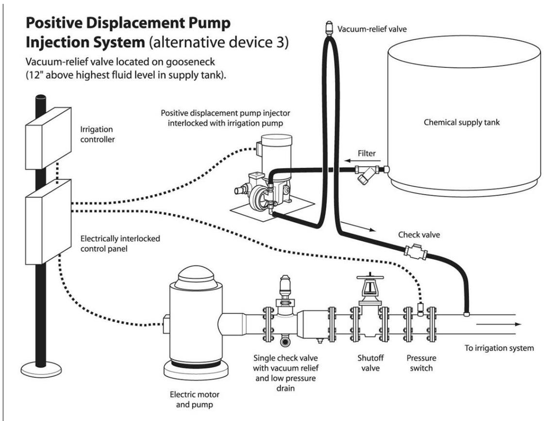
Figure 8: Vacuum relief on pesticide injection pipeline
