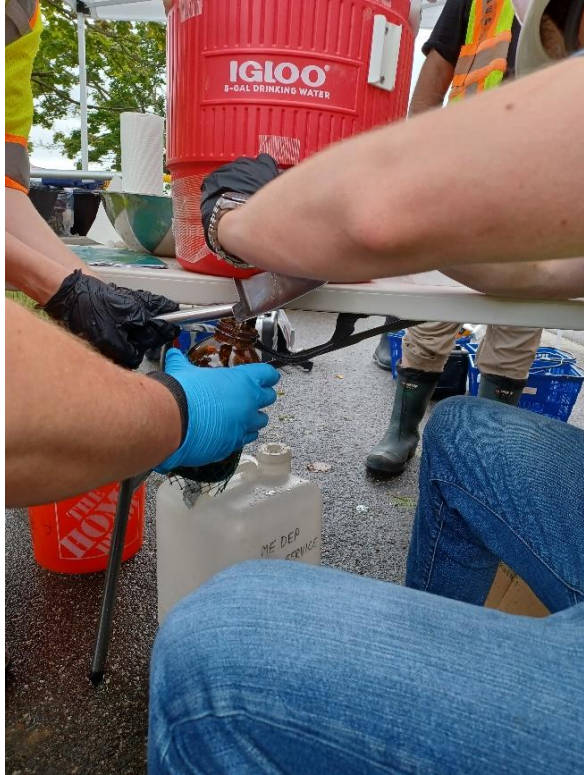
Photo 37: Equipment Blank Sample Being Collected From Sediment Trowel.
