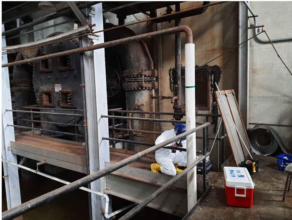
Photo 22: EF-06 Being Collected from Mezzanine with Peristaltic Pump
