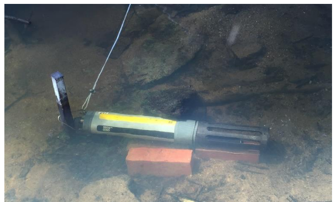
CBEP YSI 6000 series data sonde deployed in Barberry Creek – note shallow depth (August 2015)
