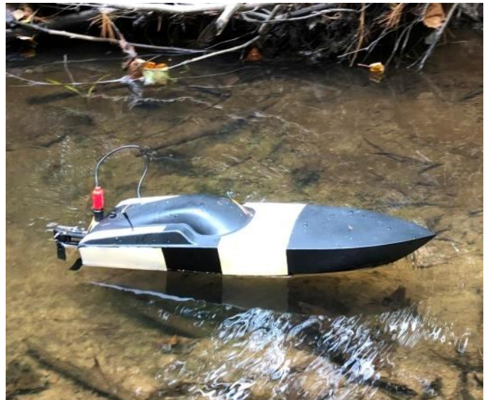
SeeBoat measuring conductivity as surrogate for chlorides in Long Creek’s South Branch (Oct. 2019)
