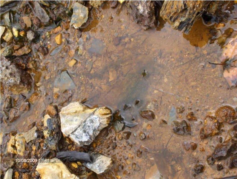
Figure 7. Photo 2 was taken in the bottom of the first pit, showing a small amount of surface water drainage after over an inch of rain the previous day. The pH of this runoff water was 2.2.
