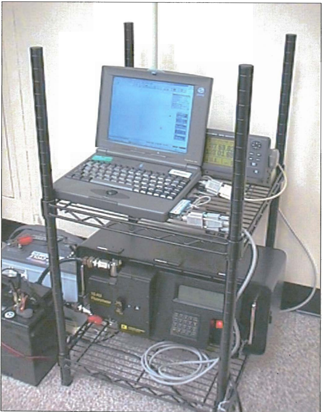
A portable computerized data acquisition and charting system used for FDA-DCP hydrography. Shown are a PC with electronic charts and ChartView Pro software; a dual serial, PCMCIA card with connections to a Turner Designs 10-AU fluorometer and a Furuno 35 DGPS; an antenna extender supporting the GPS and differential antennas; a 12V DC battery powering the DGPS, fluorometer, and PC; and a second battery powering the submersed DC seawater pump and CTD (not shown). The PC serial port is available for the CTD. A multiplexer rather than a serial card will allow logging of more than 3 instruments. The shelves provide compactness for small boats, PC access, and support for a cover.
