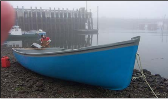
Figure 5. Typical five-ton load capacity Rockweed harvesting boat
