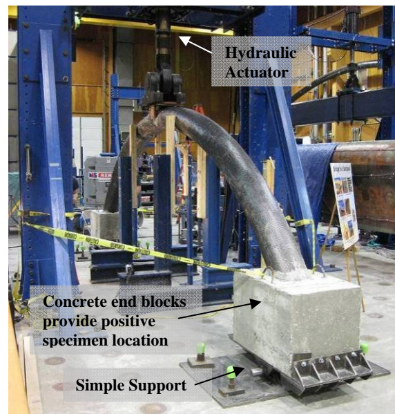
Figure 4. Arch Test Setup
