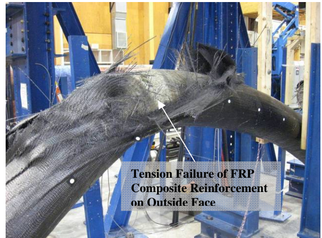
Figure 8. Arch Secondary Failure Mode
