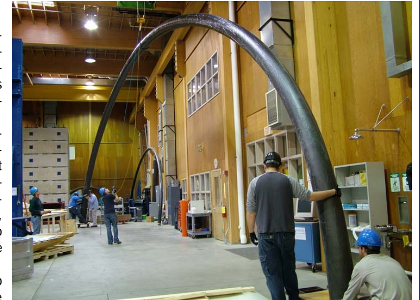
60' arch manufactured in AEWCC laboratories is light enough for two people to carry and place
