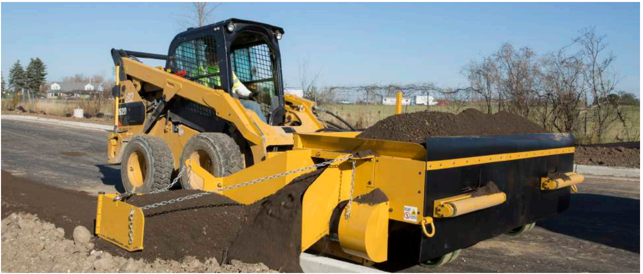
Dual discharge machine with curb backfilling option
