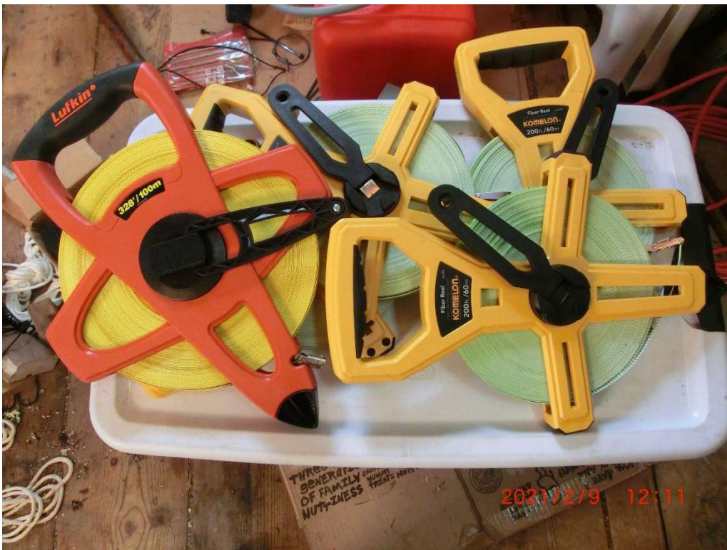
Photo 2-10 – Multiple fiberglass tape measures with metric scale on one sides
