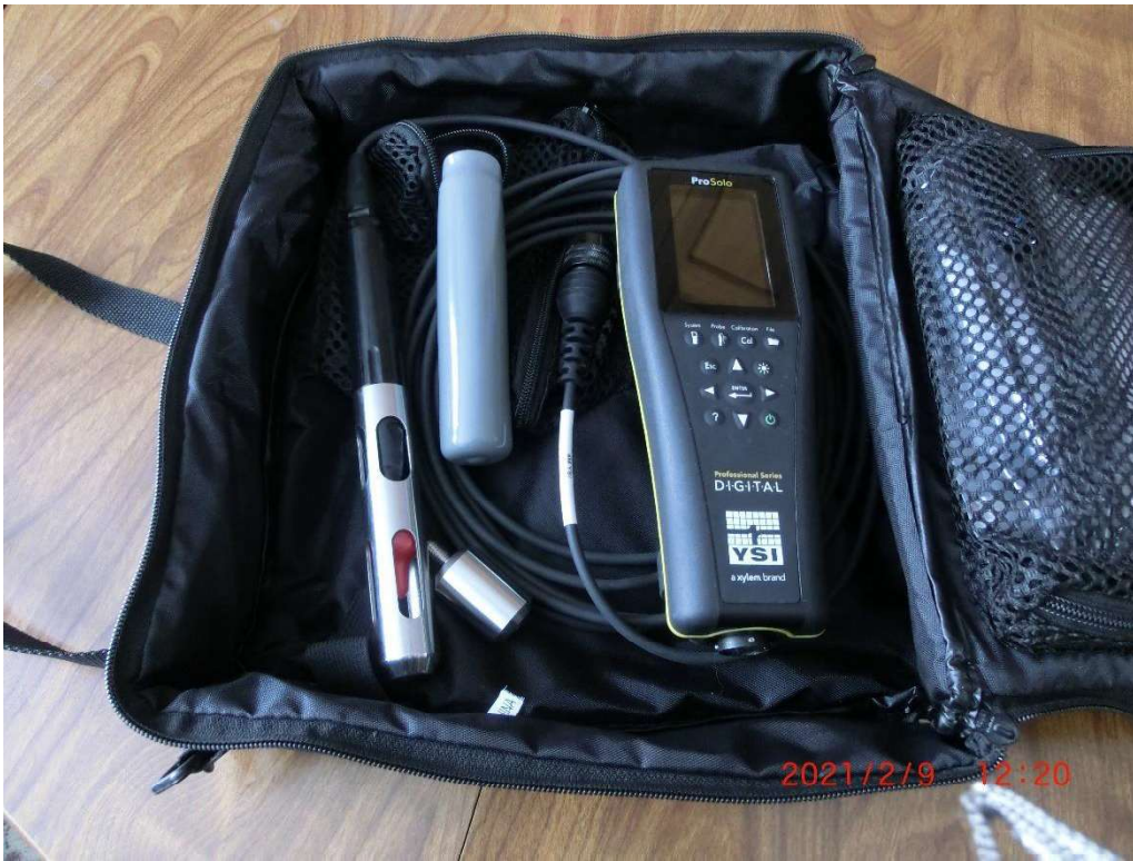
Photo 2-9 – YSI Prosolo ODOT meter with 4 meter cable & DO/T probe
