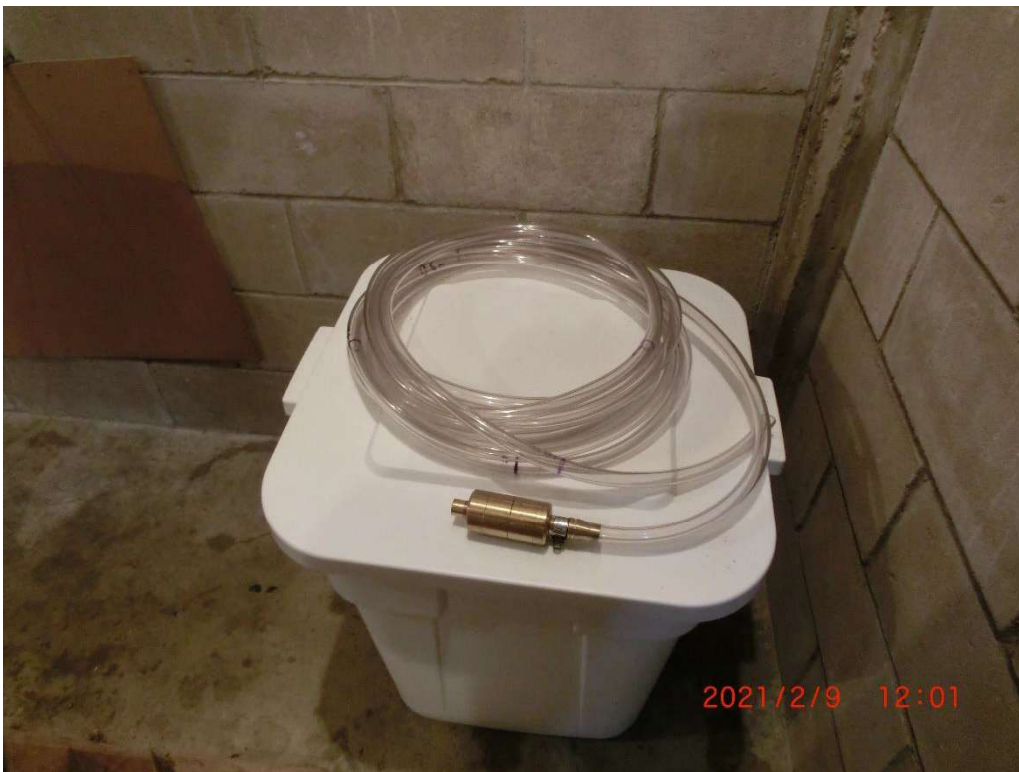
Photo 2-4 – 10 meter epilimnetic core sample tube per MDEP specs
