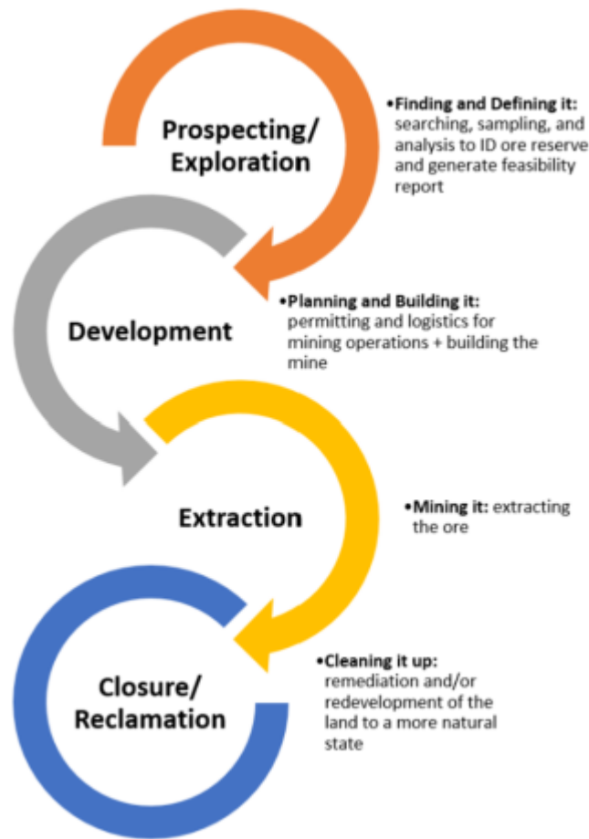
Figure 1. The Life Cycle of a Typical Mine. Source: University of Arizona Superfund Research Center
