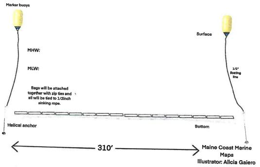
This cross-section view depicts bags being attached end to end in rows running the length of the lease. There may be collection boxes at the deepest end and there may be a 2' wide row for walking in the center of the row. (See overhead view option 1) Soft bags may potentially be covered by 4' wide predator netting.
