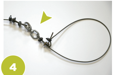
2 Place the stop on the mark and close the loop.
