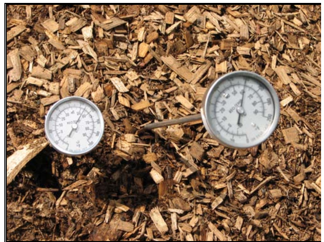
Thermometers are used to monitor compost pile temperatures. Goal is to keep the temperature between 110 to 145 degrees F for optimal composting.
